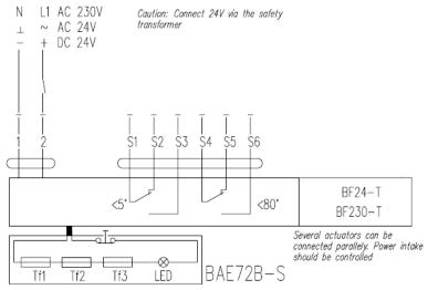
**Connection diagram for the BF24-Tand BF230-T actuators**
