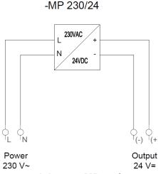
Connection diagram for transformer module type MP230/24
