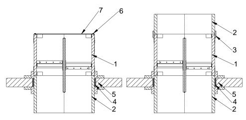
Installation of damper in rigid floor - above the rigid floor
