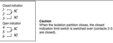
Electric connection diagram of WK1 and WK2 limit switches
