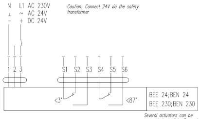
connected parallely. Power intake should be controlled
