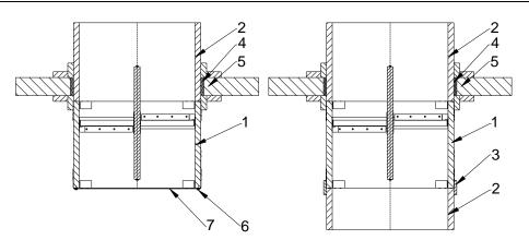
Installation of damper in rigid floor - below the rigid floor
