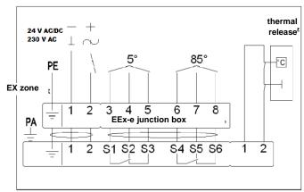
Wiring diagram for EXBF actuators
