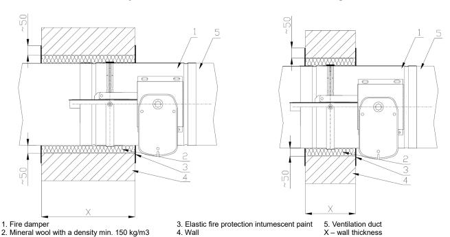
The minimum depth of filling with mortar for the length of the body of the device.
