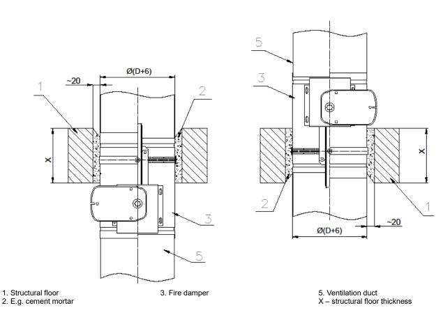
Installation of the mcr FID PRO fire damper with an electric mechanism in structural floors using mortar
