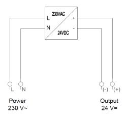
Connection diagram for transformer module type MP230/24
