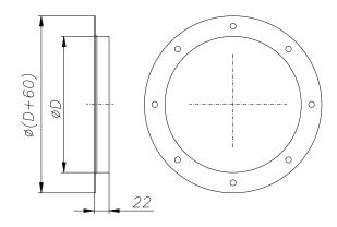
Flange dimensions in the case of the flange version of the fire damper. Spacing and quantities of openings according to EN 12220 (dimensions of flanges with circular intersection for comfort ventilation purposes).
