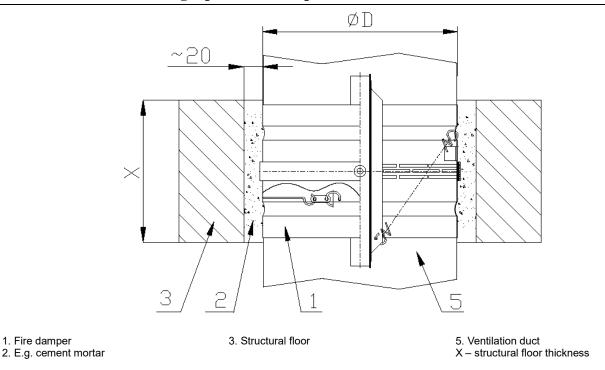
Installation of the mcr FID PRO fire damper with a spring mechanism in structural floors using mortar
