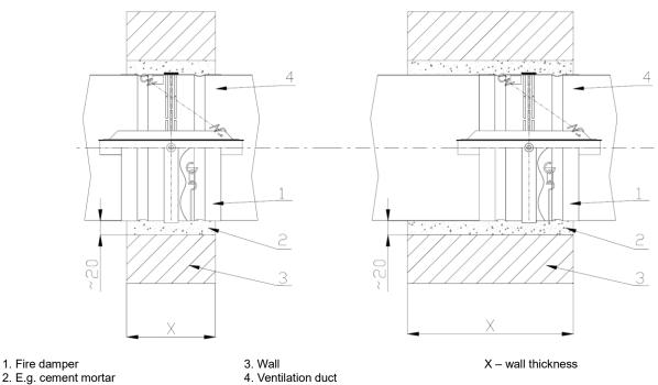
The minimum depth of filling with mortar for the length of the body of the device.
