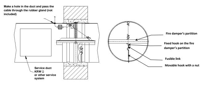
Separate limit switches of fire dampers – for the RST manufacturing version
