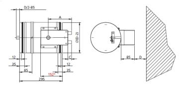
mcr FID PRO fire damper with RST/KW1
