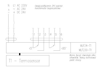
Note: MLF actuator cables are not marked with symbols. It should be connected based on the colors of the wires.
