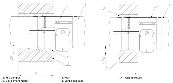
The minimum depth of filling with mortar for the length of the body of the device.
